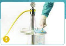
If the suction is foreseen with one FLOVAC® container only, close firmly and carefully the TANDEM connecting port by using the specific plug provided.
